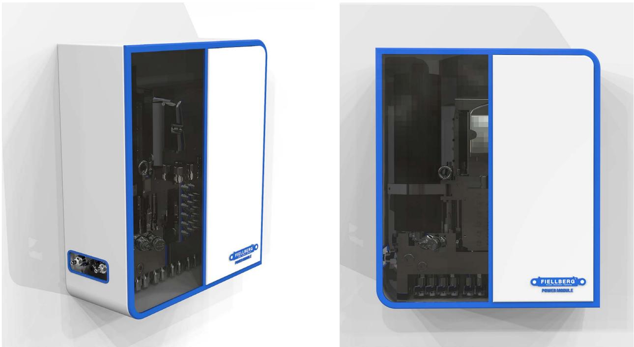
Fiellberg Oy has built a proof of concept (PoC) device highlighting the benefits of the digital hydraulic multi-pressure actuator approach. The key concept of the technology is to avoid throttling losses associated with traditional valve controlled hydraulics. Another main benefit is the fact that the device consumes only small average input power while creating significantly bigger peak powers from its local energy storage, which is a hydraulic accumulator.
